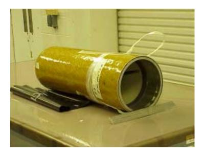
FIGURE 4. Eight-inch-diameter Test Bottle (IM Motor Without Dummy Nozzle) Loaded With MPE Propellant
