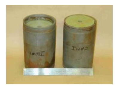
FIGURE 3. Analog Motors Used for Verification of Low-temperature Storage Capability.
