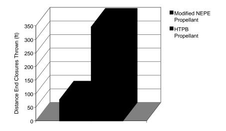
FIGURE 2. Results of Slow Cookoff Testing of 8-inch-diameter, 120-lb Steel-cased Rocket Motors Containing Modified NEPE and HTPB Propellants.
