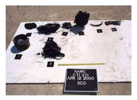
FIGURE 6. Material Recovered Following Slow Cookoff Testing of IM Motor.
